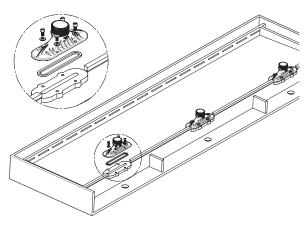
Ensure that the sealing gasket is correctly fitted into the recess on the funnel and tighten the 4 fixing
