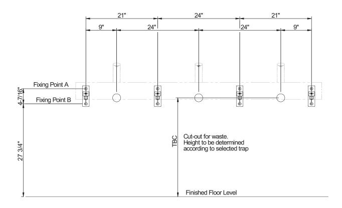
The fixing centres given in the table are only a guide, so can be moved within a tolerance of +/- 2" to suit the wall conditions and the position of the waste outlet.
